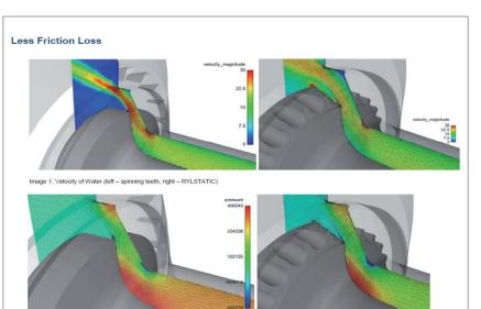
Image 2: Static Pressure distribution (left – spinning teeth, right – RYLSTATIC)
